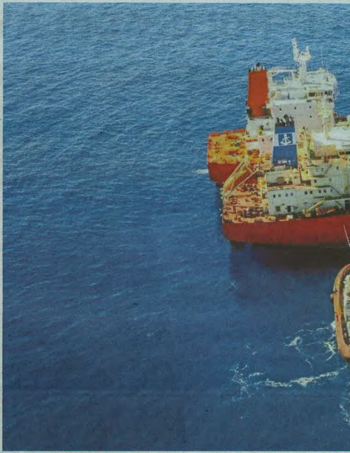
SHAPE OF THINGS TO COME: Ammonia is transferred from Mitsui OSK Lines' 35,200-dwt LPG carrier Green
